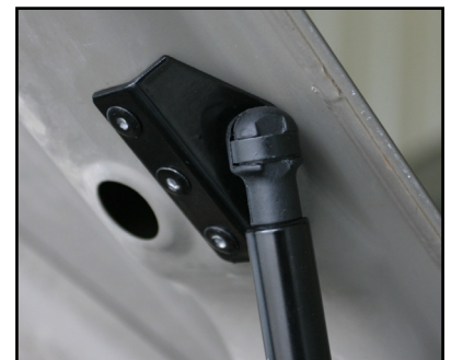
C. Slide clip over ball-stud to lock end-fitting
