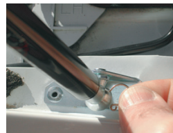
A. Insert clip into hole.
