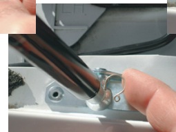
B. Slide clip down till it stops.
