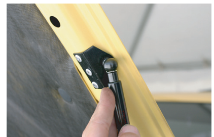
Rotate clip until it snaps onto shaft.
