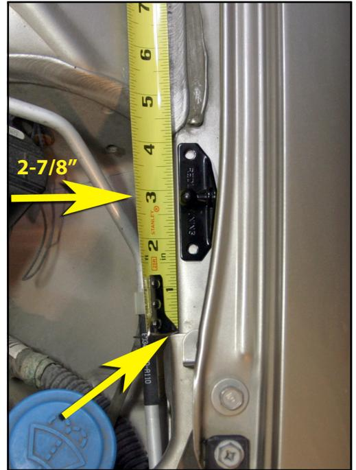
**Step 10 - Attach the right side of the bracket to fender.**
