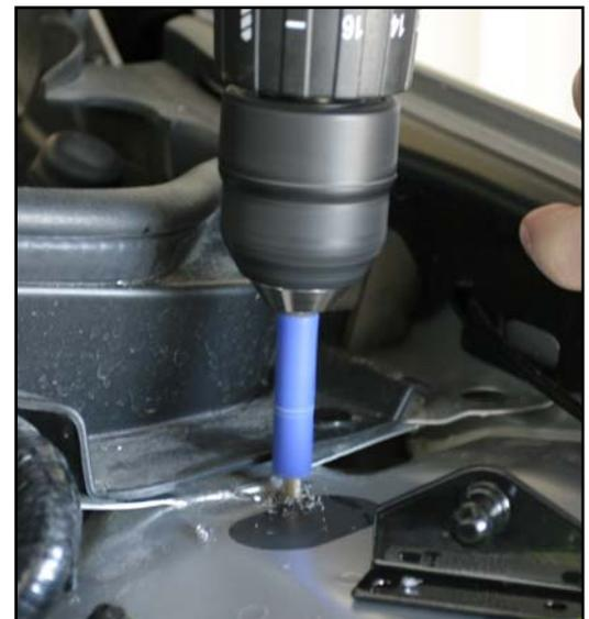
**Step 11 - Attach the right end of the bracket to fender.**
