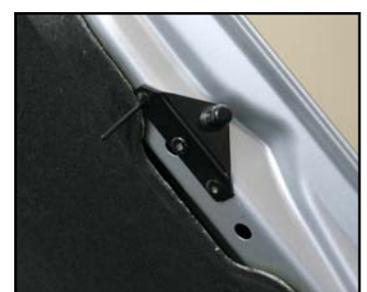
**Step 8 - Repeat steps 3-7 and install the passenger side hood bracket.**
