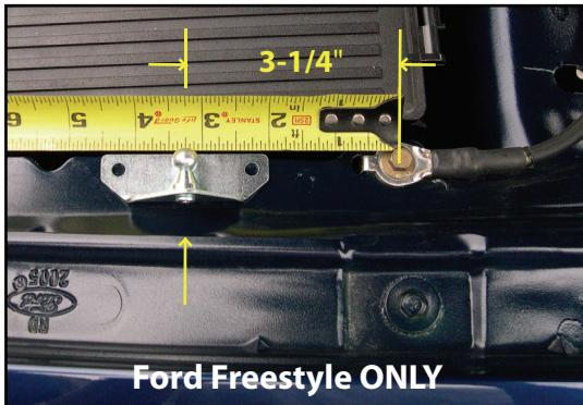
**Ford Freestyle ONLY** - Place a mark **3-1/4"** down from the ground strap's bolt centerline as shown below. This mark will be used to align the centerline of the bracket. The mark should be placed on the inside edge of the inner fender...the lower arrow shows where to place the mark.
